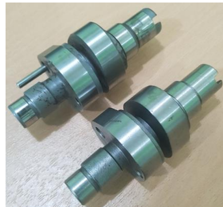
Fig. 2. Camshaft for automatic motor cycle 125 cc used in this research.
